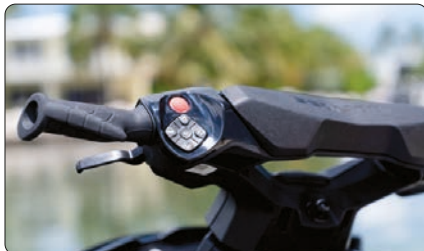
iDF - Intelligent Debris Free system An innovative, industry-first system that allows you to free your pump of weeds and debris with intuitive handlebar-activated controls.
