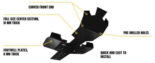
Our Plastic Plates glide smoothly and silently over obstacles, offering great protection in rough terrain. Made of abrasion-resistant thermoformed High Molecular Weight Polyethylene (HMWPE).
