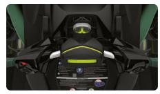
Hydraulic Steering Damper and Redesigned Steering Column
