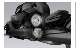
**AUTOMATIC TRANSMISSION (CVT)** No need to worry about changing gears as your continuously variable transmission will find the accessible performance, while the 3-cylinder perfect combination of performance and fuel efficiency for you.
