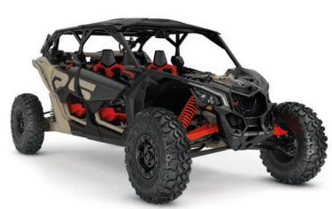
149 kW (200 hp\*), Rotax® ACE (Advanced Combustion Efficiency) 900 cc Turbocharged Triple-cylinder engine, liquid cooled with integrated intercooler and high-performance air filter
